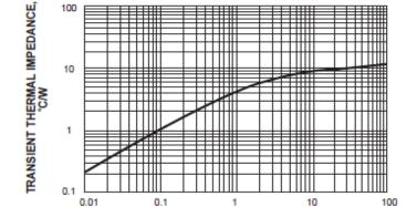
FIG. 6-TYPICAL TRANSIENT THERMAL IMPEDANCE
