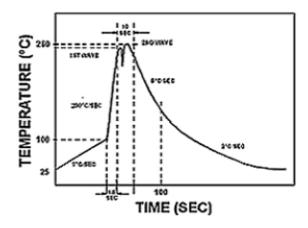
The Recommended solder Profile For Devices with Pb-free terminal plating used with leaded solder, or for devices with leaded terminal plating used with leaded solder
