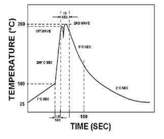
The Recommended solder Profile For Devices with Pb-free terminal plating used with leaded solder, or for devices with leaded terminal plating used with leaded solder
